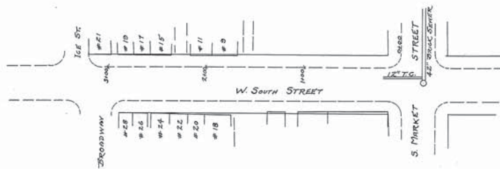
PLAN OF PROPOSED SEWER WEST SOUTH STREET FREDERICK MARYLAND SCALE - HORIZ. 1" = 40' VERT. 1" = 4' SEPT. 18, 1928
